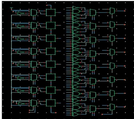
**Figure 3: Schematic of the Proposed ALU**
