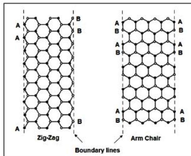
Figure 2: Lattice Structure of AGNR and ZGNR
