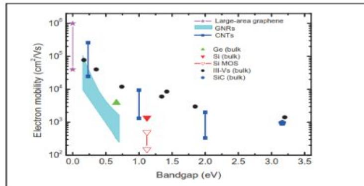
Figure 1: Electron Mobility Vs. Band Gap for Different Materials
