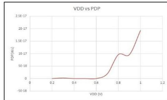
**Figure 5: VDD vs. Power Delay Product of 2x1 MUX**
