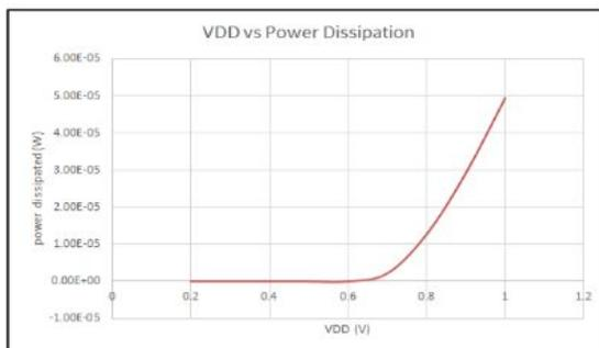
**Figure 5a: VDD vs. Power Consumption of 2x1 MUX**
